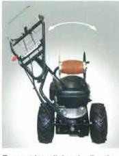
Prompt handlebar inclination in several position on both the sides
