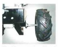
Wheel base may be widened in step to set the distance of the lain loop from the border (25 - 27 - 39 - 31 cm).
